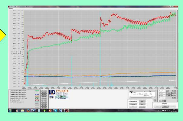
Lysimetric set also includes a complex automatic weather station for measuring relative humidity, wind direction, wind speet, globally radiation, air temperature and precipitation.
