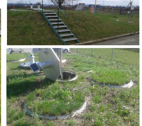
It is a container set of five lysimeters with different soil monoliths of cylindrical shape with area 1m<sup>2</sup> and depth 2.5 m with groundwater regulation.
